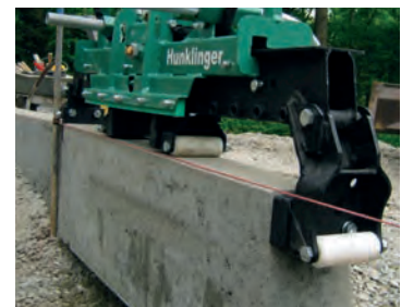
Lay against a guideline Exact lateral laying through long-sided grabbing
