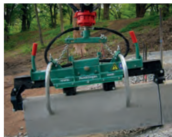
Inclination settings Inclined laying of kerbstones
