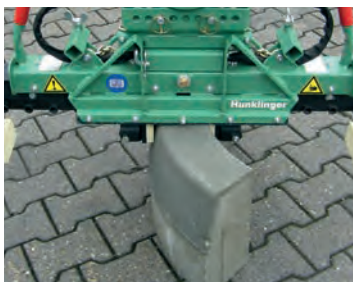
Grabbing crosswise Laying radial kerbs or picking up straight kerbs
