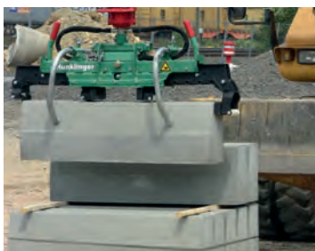
Assistance-free pick-up Operator picks up kerbs from the pallet on his own
