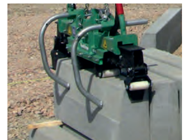
Support bow Help for quick and easy pick up of kerbs
