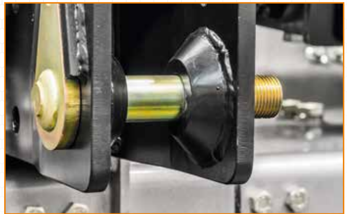
Conical hitch for 3-point linkage arms.
