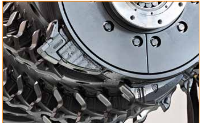
Forged tooth holders with lateral protection.
