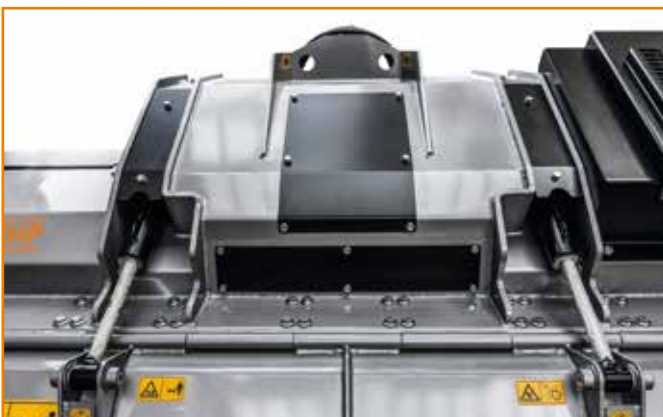
Access points to facilitate the maintenance.
