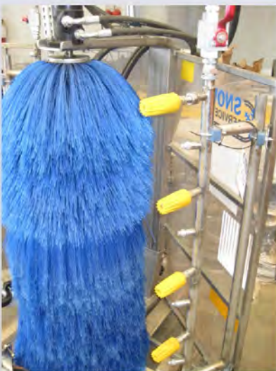
Stainless steel bar with special rotary nozzle for high pressure washing.
