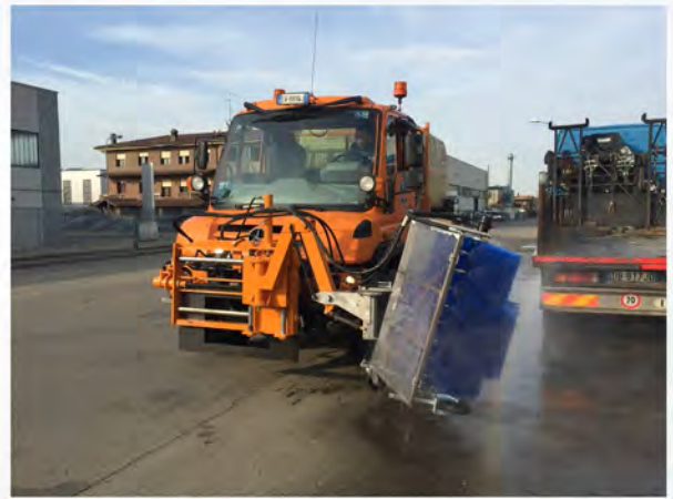
Brush ø 800 mm with protection cover in ppl , mechanical inclination of the brush (to adapt at the various type of washing work).
