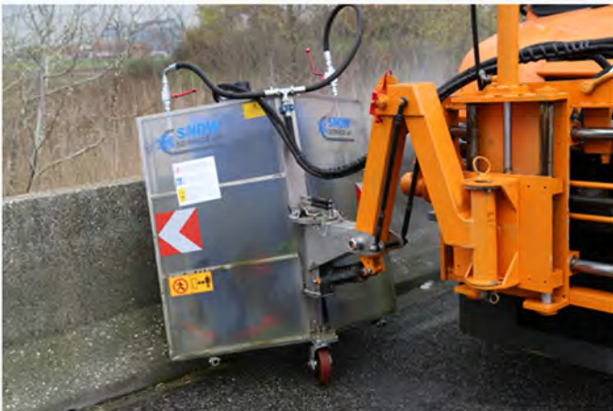
Brush ø 800 mm with protection cover in ppl , mechanical inclination of the brush (to adapt at the various type of washing work).
