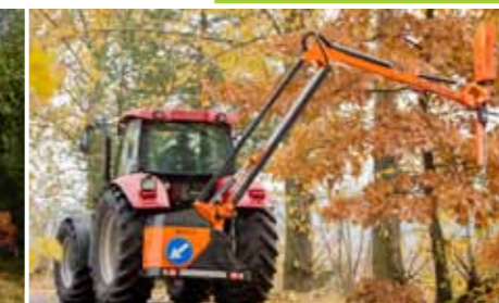
WWT600P - parallel system for head angle keep when adjusting arm
