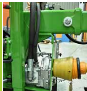
Multiplier powered by tractor PTO
