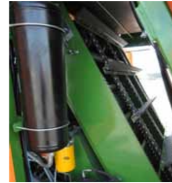
Scraper conveyor transporting waste to the hopper.
