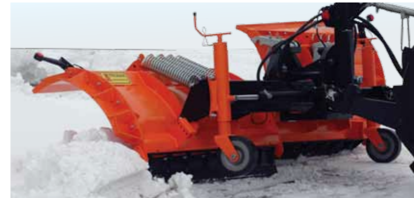
Segmented mouldboard with spring safeguard.
