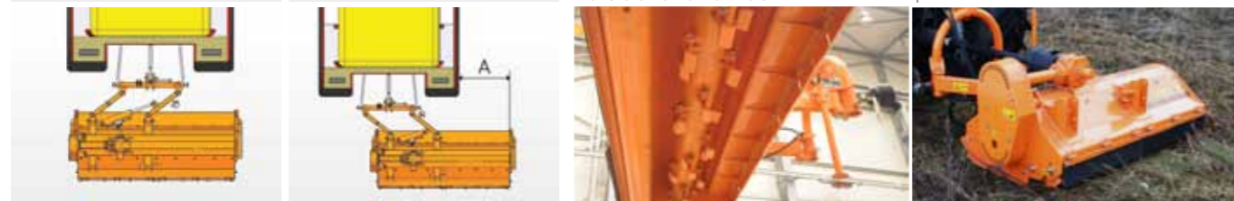
Regulation of mower position (parameter A - see table)
