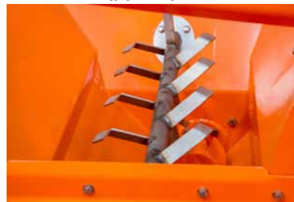
Additional mixer facilitates aggregate breaking
