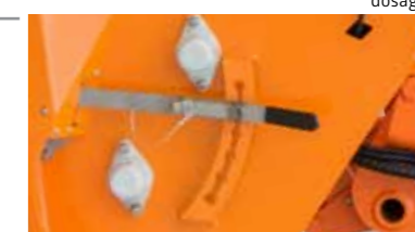
Aperture adjustment to set the spreading dosage.
