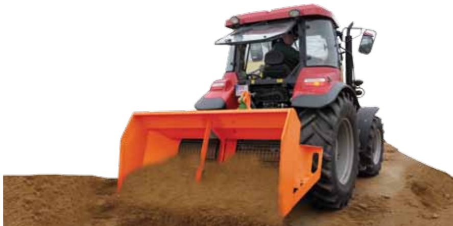
Additional mixer facilitates aggregate breaking
