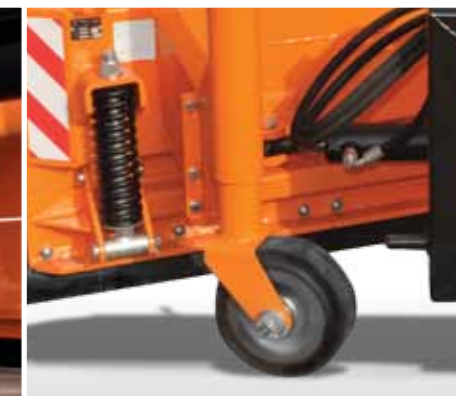
Spring safeguard (extendable blades)
