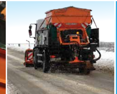
PT series vehicle-mounted sand spreader with axle drawn by carrying vehicle.
