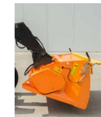
Aperture adjustment to set the spreading dosage.
