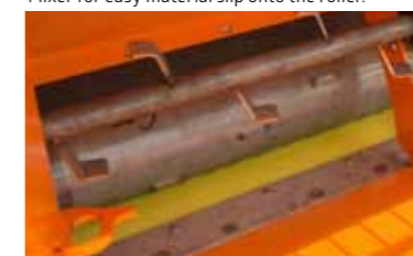
Mixer for easy material slip onto the roller.
