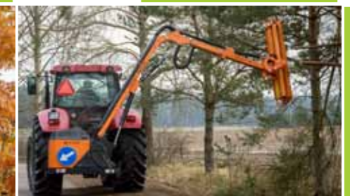
WWT700T, WWT800T - Long arm reach is provided thanks to hydraulic telescopic sliding
