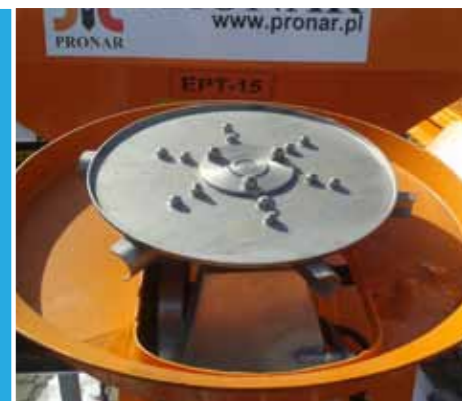
Stainless steel spreading disk.
