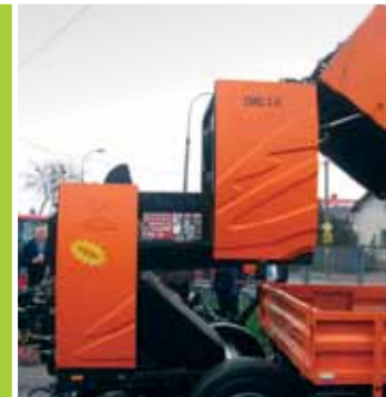
Hydraulic hopper dumping system.
