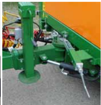
Hydraulic drawbar articulation
