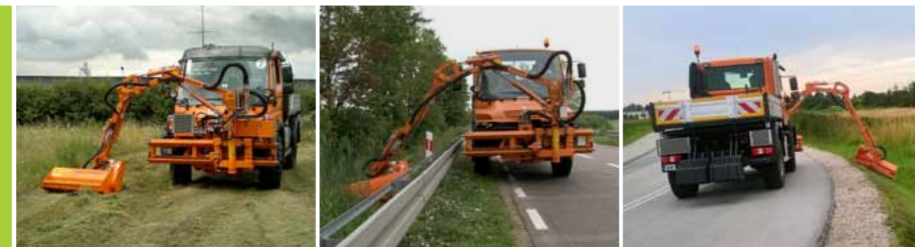
WWP500U multifunction arm with GK10 mowing head on Unimog U500
