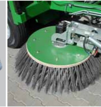
Hydraulic adjustment of rotary disc brush position.
