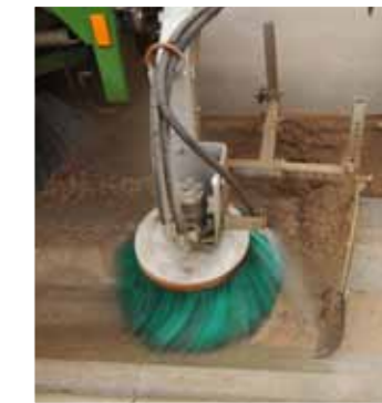
Hydraulic brush for gutter cleaning
