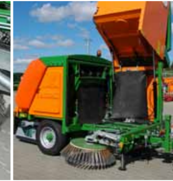
Hydraulic hopper dumping system.
