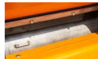
Working roller with slats dispense the material on the road.
