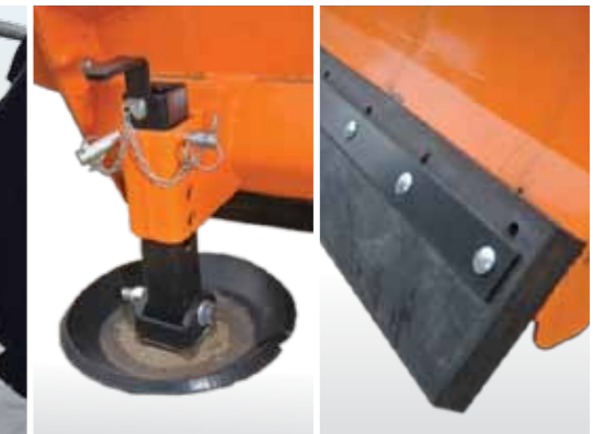
Slides made of abrasion-resistant steel. Rubber blade
