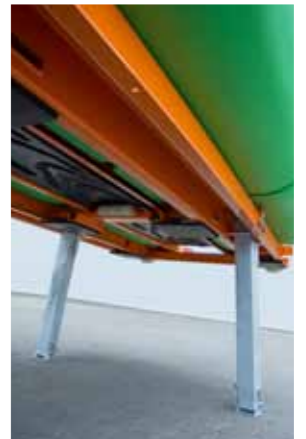
RORO (Roll-on / Roll-off) system for easier loading of PT70 spreader on the carrier bed
