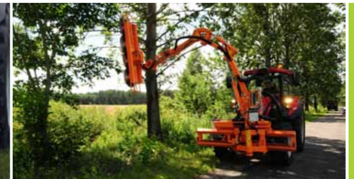
WWP600 multifunction arm with GP200 saw for branch cutting.
