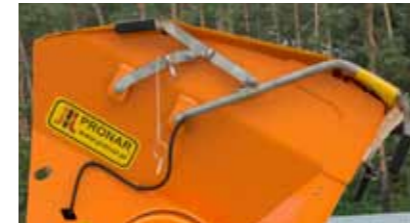
Canvas cover with frame protects the material from snow and rain.
