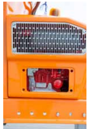
Combustion engine with 1000 ccm capacity and 16.2kW power
