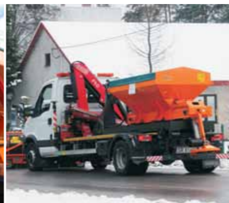
Capability of aggregation with a hook loader.
