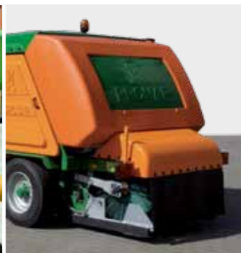
1150 litre water tank and roller brush.
