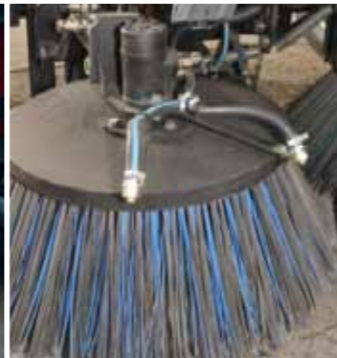
Spraying nozzles in front of rotary disc brushes
