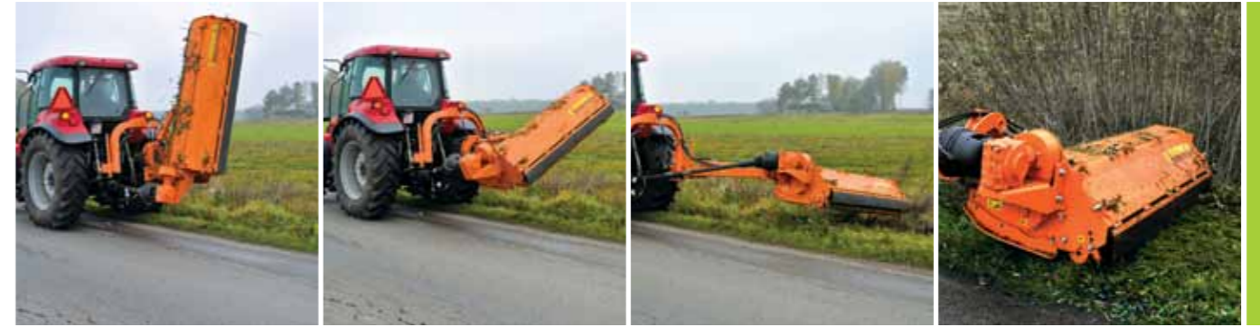
Mower works on right side of the tractor, vertical rest position
