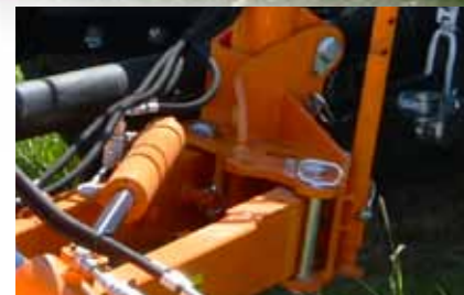
Mechanical protection prevents damage when hit an obstacle
