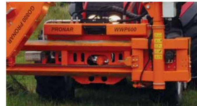
WWP600 multifunction arm – hydraulic movement of working arm over guide rail.
